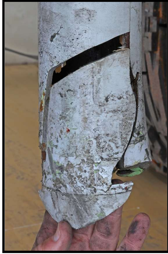
Figure 45. Detailed view of Upper Drag Strut- Fracture.
