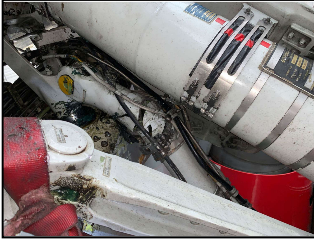
Figure 7. Photo of MLG-Upper Drag Strut.
