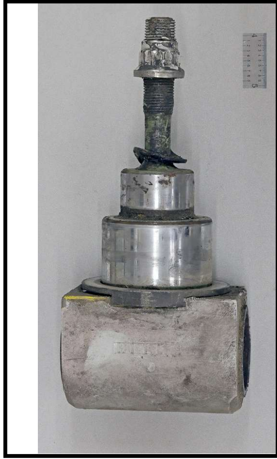
Figure 15. Overall view of R/H MLG- Tee Bolt. Note: Nut is still attached and washer is deformed.
