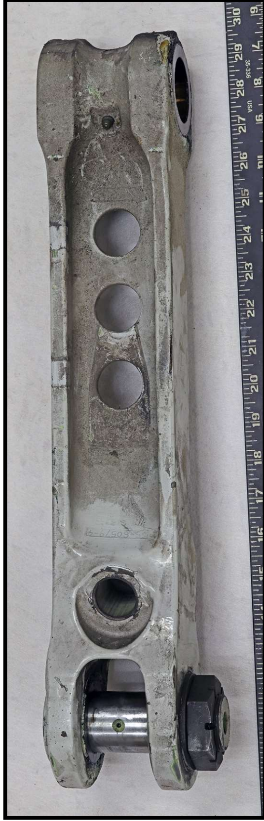
Figure 80. Overall view of Lower Drag Strut (FWD Side).
