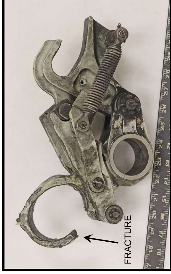
Figure 88. View of R/H MLG- Side Strut/Bell Crank Link Fracture.
