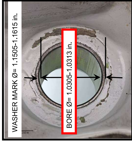
Figure 81. Overall view of Lower Drag Strut- Tee Bolt Bore Diameter.
