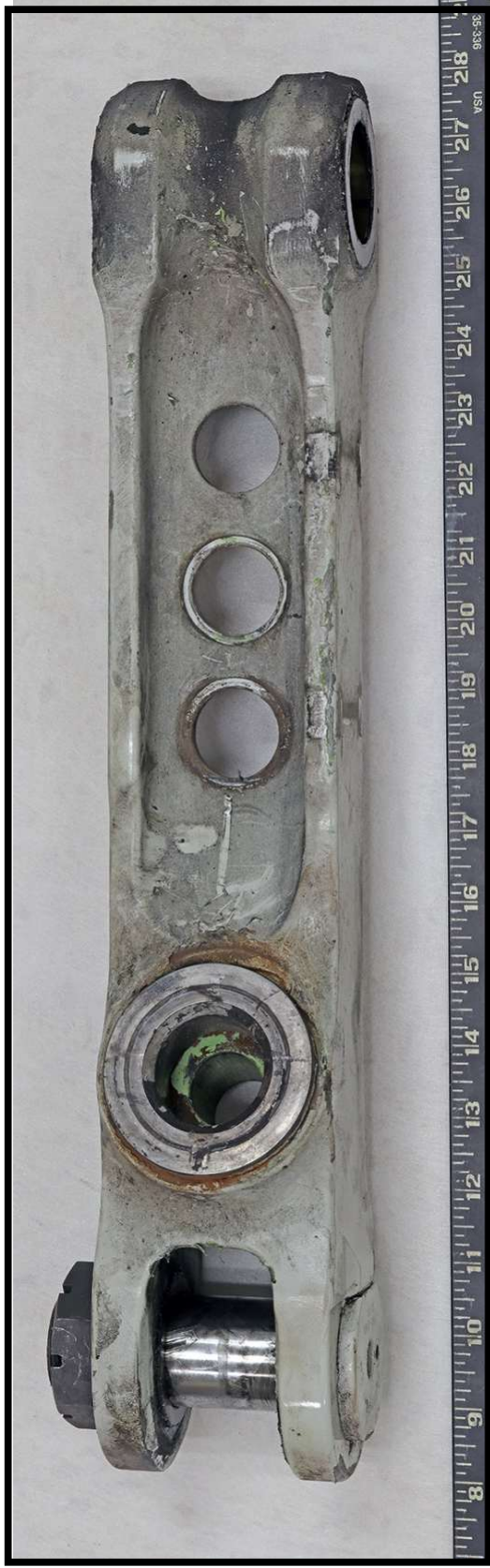
Figure 75. Overall view of Lower Drag Strut (Aft Side).
